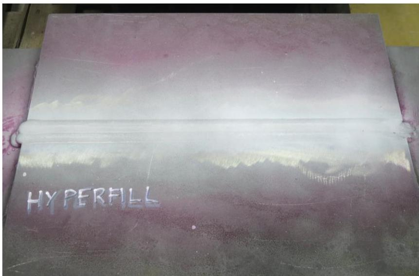
Fig. 3.2.1 – Liquid penetrant inspection on HyperFill™ butt joint
