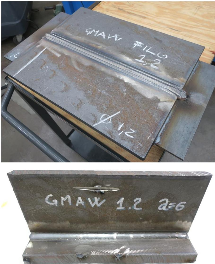
Fig. 2.2.5 – Joints realized with GMAW process
