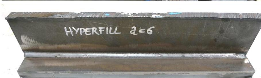
Fig. 2.2.4 – Joints realized with HyperFill™ process
