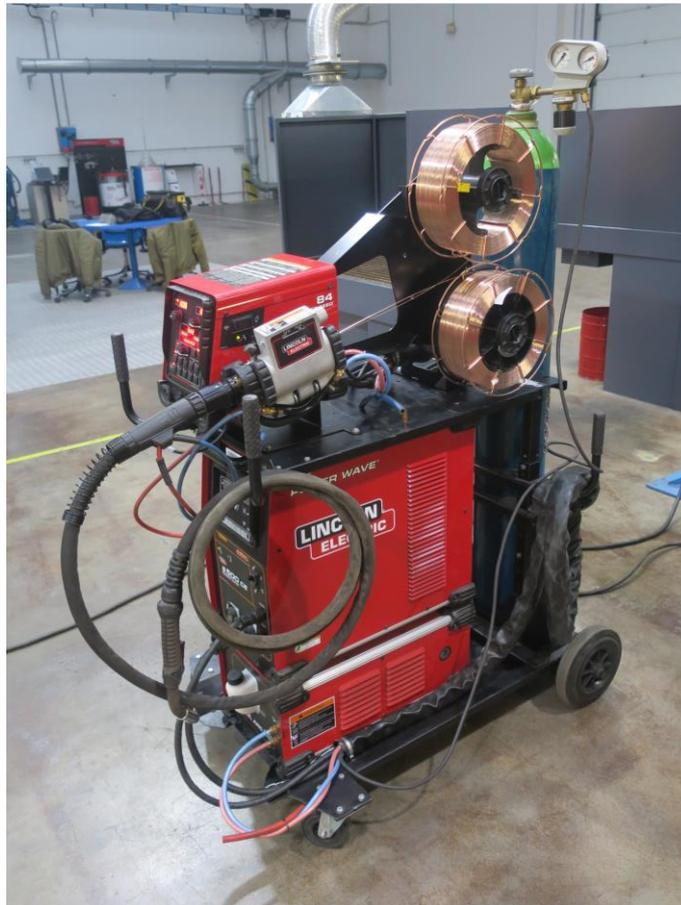
Fig. 1.1 – Welding generator and equipment for HyperFill™ technology
