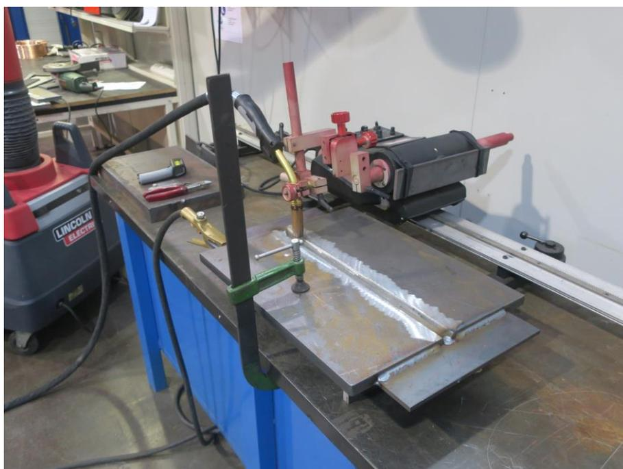
Fig. 2.2.1 – Fit-up of the butt joint
