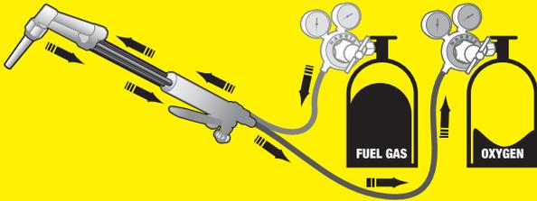
2. Both cylinder valves are closed with unequal pressures in the regulators and the torch valves closed. If the operator opens both torch needle valves simultaneously to bleed off the oxygen and fuel gas, typically higher pressure oxygen may reverse flow into the typically lower pressure fuel gas hose, regulator and upstream gas supply.
