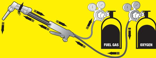
3. The operator opens both torch valves and attempts to light both gases at once. If more oxygen is flowing than can flow through the tip, the system is back-pressured and oxygen can reverse flow into the fuel gas hose and regulator.
