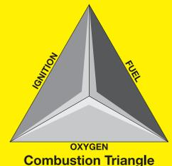
On the other hand, you can't have a fire without fuel. An automobile won't run on an empty gas tank. Finally, a combustible mixture isn't dangerous until it's lighted. Mixed gases in a hose or regulator aren't hazardous until they're lighted. This ignition can occur several ways.
