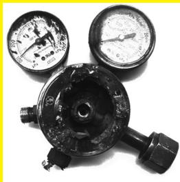
The subsequent explosion is violent and injuries come from both the flames and the disintegrating metal.
